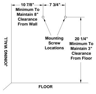
Figure 3 - Mounting Screw Locations
